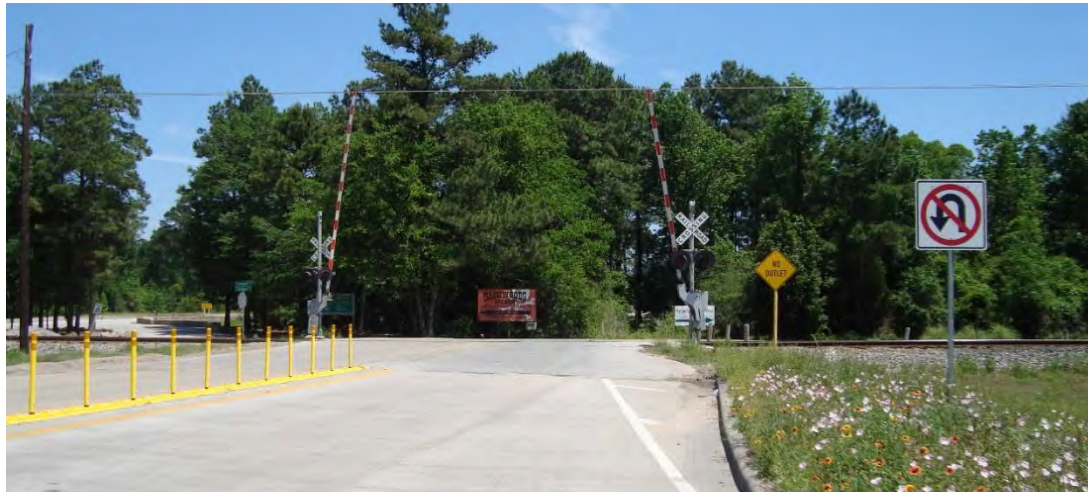
Figure 7.3: At-Grade Railroad Crossing
